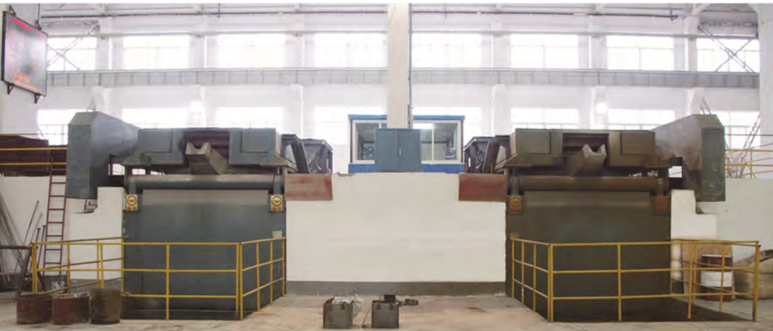
2台18吨中频感应熔化炉 Two 18T MF Induction Melting Furnace 2台15吨自动加料配料系统 Two 15T Automatic Ingredients Feeding Machine
