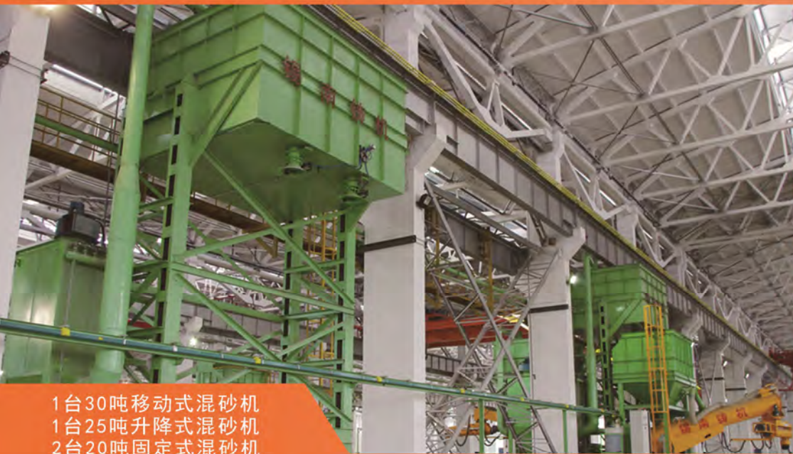
One 30T Travelling Double Arm Sand Mixer One 25T Lifting Double Arm Sand Mixer Two 20T Fixed Double Arm Sand Mixer Two 10T Fixed Double Arm Sand Mixer
