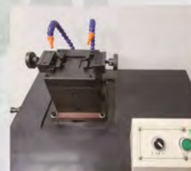
冲击试样缺口电动拉床 Electric Broaching Machine For Notches Of Impact Specimens
